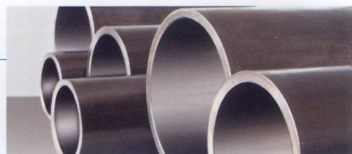
Our cylinder tubes are produced by cold drawing, hot rolling and cold rolling processes. The production of seamless cold drawn tubes (SCD) is carried out by a continuous cold drawing line. The cold drawn tubes (DOM) are produced by a cold drawing line. The hot rolled tubes (HRT) are produced by a hot rolling line. The smooth bore tubes (SSID) are produced by a cold rolling line.
